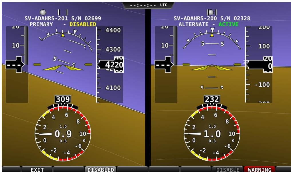
Figure 57 – ADAHRS Cross-Check Comparison (one ADAHRS disabled)
