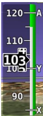
Figure 14 – Example V speeds
