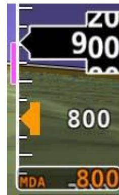
Figure 20 – MDA Bug Detail
