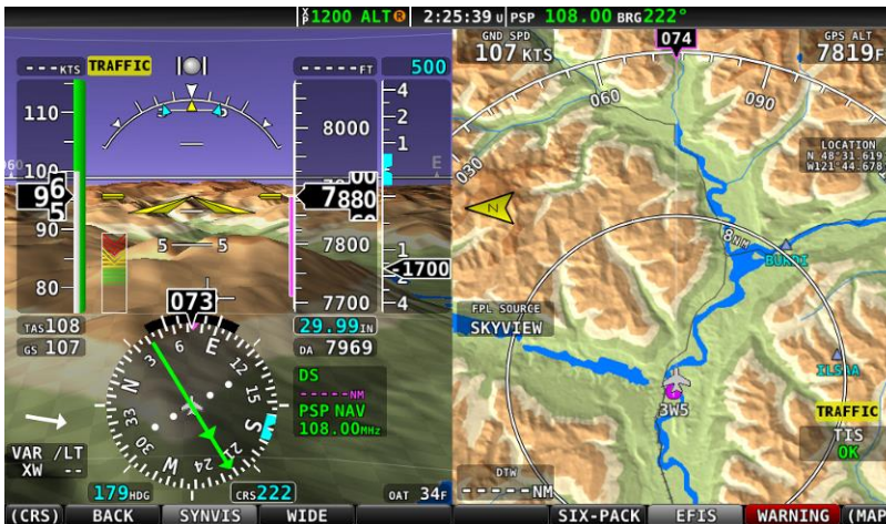
Figure 44 – SkyView Synthetic Vision Normal View
