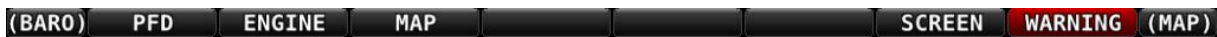
Figure 231 - Message Notification Area above button 8 (2nd from right), showing a Warning Notification
