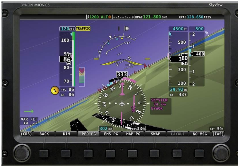
Figure 43 – SkyView Synthetic Vision View with Runways
