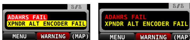
Figure 233 – Unacknowledged (left) and Acknowledged (right) Alarms
