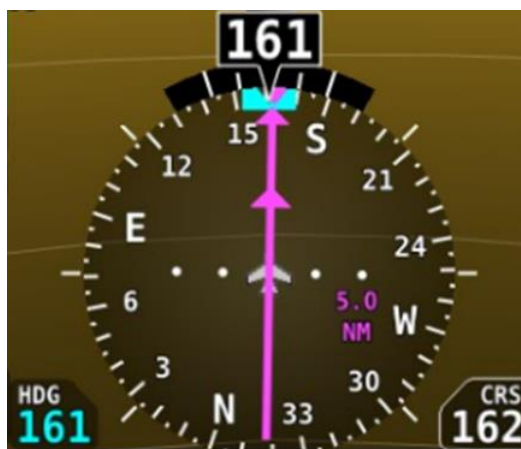
Figure 26 – HSI Example - Localizer
