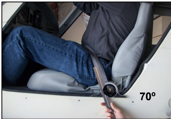
Current configuration: Seat-back in mid-position
