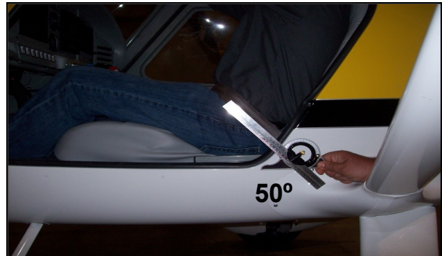
Retrofit (new) configuration: Seat-back in aft position
