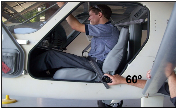
Current configuration: Seat-back in forward position
