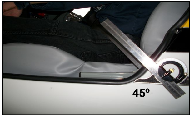
Retrofit (New) configuration: Seat-back in forward position
