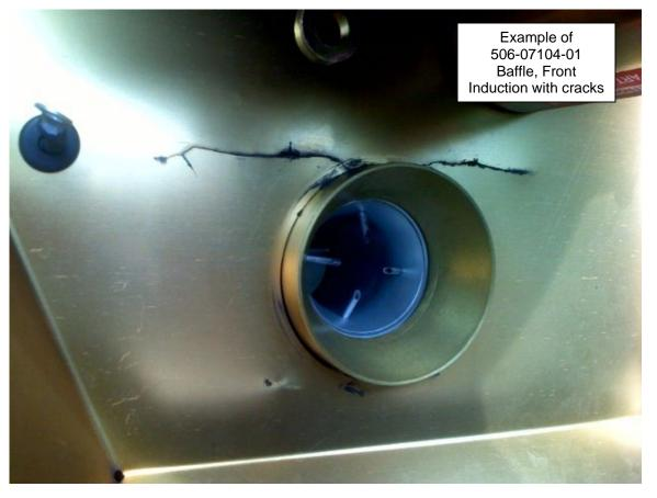
Allowing the stress cracks to propagate may eventually result in a baffle leak large enough to possibly affect engine cooling.
