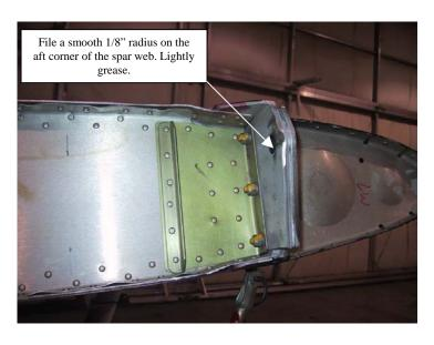
3) Be sure to have the head of the aft spar bolt at the pivot fitting facing aft. This will provide clearance from the cage and drain pans. Also be sure to torque the bolt firmly to minimize racking of the spar in the fitting.
