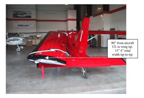
Folding the wings to a tip-to-tip dimension of 13' 4" leaves the flap tracks just outside of fuselage contact. This may be enough to gain optimization of shared hangar space for those not concerned with attaining a road-legal width of 8' 6".
