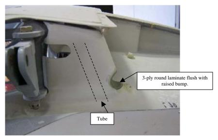
B) The upper trailing edge of the wing will slightly make contact with the upper, aft edge of the hatch cover joggle. Carefully swing the wing to determine the contact point and relieve it with a 1" drum sander.
