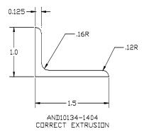
If you have received the incorrect angle (TMS 60-214) with your kit, please contact Glasair Aviation for replacement material at no charge if complied by August 1, 2005. The part number for the replacement material is the same (100-0640-009).
