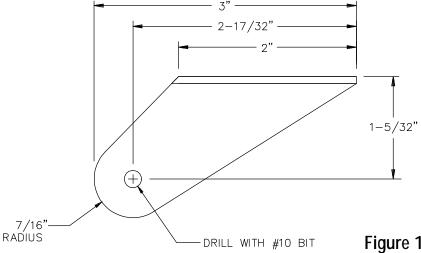
Figure 1: Dimensions for New-Style Trim Tab Control Horn
