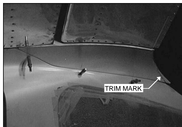
Figure 146: Fitting the Lower Hatch Half Trailing Edge
