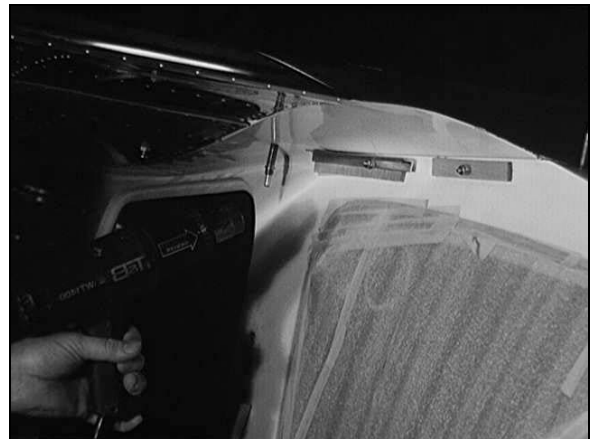
Figure 154: Adjusting the Lower Hatch Joggle
