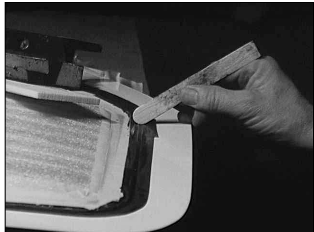
Figure 176: Cleaning Up Excess Resin on the Outside Surface
