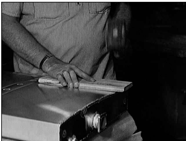
Figure 96: Tapping the Bulges Out of the Fuel Tank
