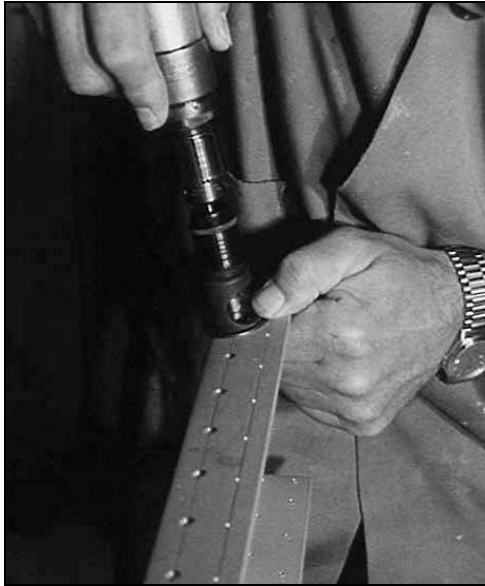
Figure 58.1: Countersinking the Spar
