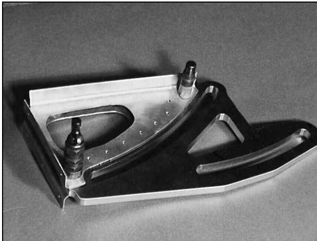
Figure 74.2: Flap Track Assembly
