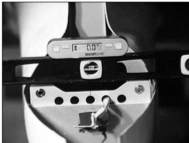
Figure 93: Leveling the Stabilizer Attach Bracket
