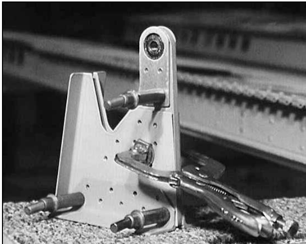
Figure 59.1: Assembling the Aileron Hinge
