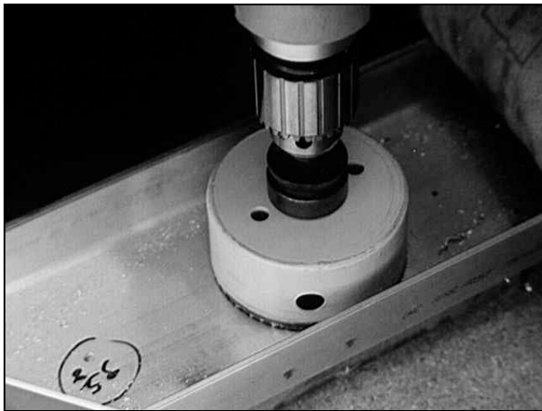
Figure 7.1: Drilling the Lightening Holes
