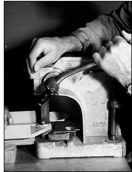
Figure 26.1: Pressing in the Wing Attach Bushing
