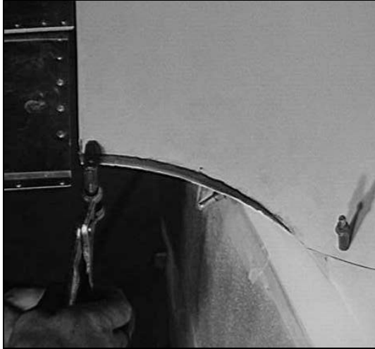
Figure 150: Clamping the Hatch Trailing Edge
