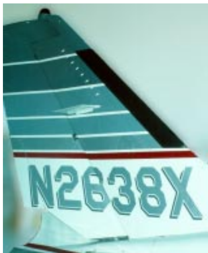
Figure 9 — VGs are applied to both sides of the vertical tail!
