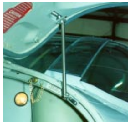
Figure 12 — BLR's Spring Thing installed on the nose compartment door of my 310. I also have two more installed in the wing lockers.
