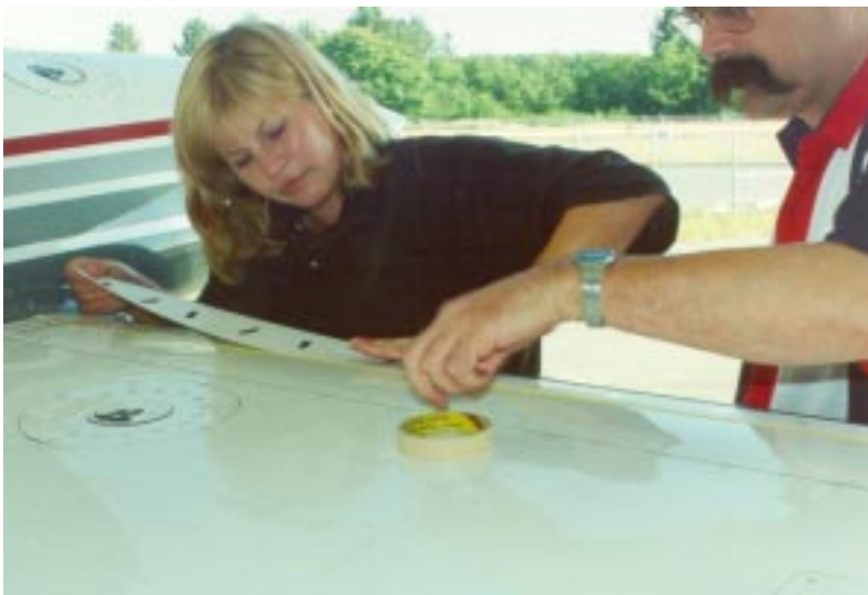
Figure 2 — Jean and Jay apply wing template using a taut string.
