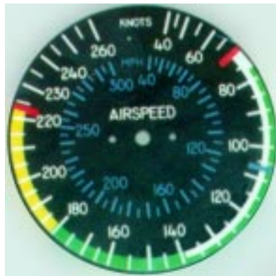
Figure 8 — My re-marked airspeed dial. Vmc is now below Vs.
