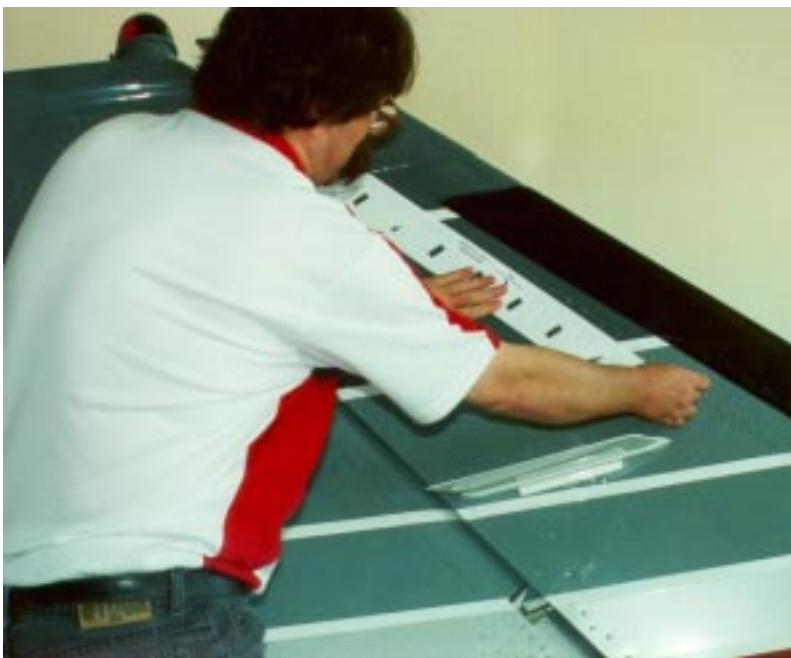
Figure 3 — Jay installs vertical stabilizer template along a skin lap. (That giant VG below Jay's right arm is my VOR antenna!)
